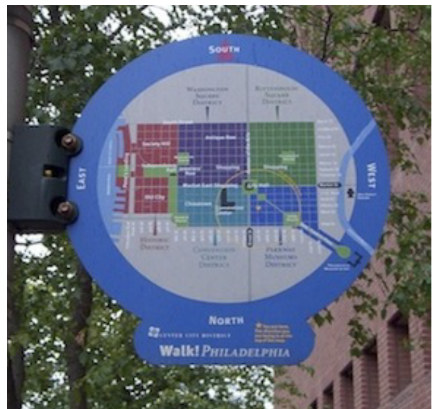
Figure 4.20 Pedestrian wayfinding map from Philadelphia. Note that the map orientation changes depending on the direction the pedestrian is facing.
