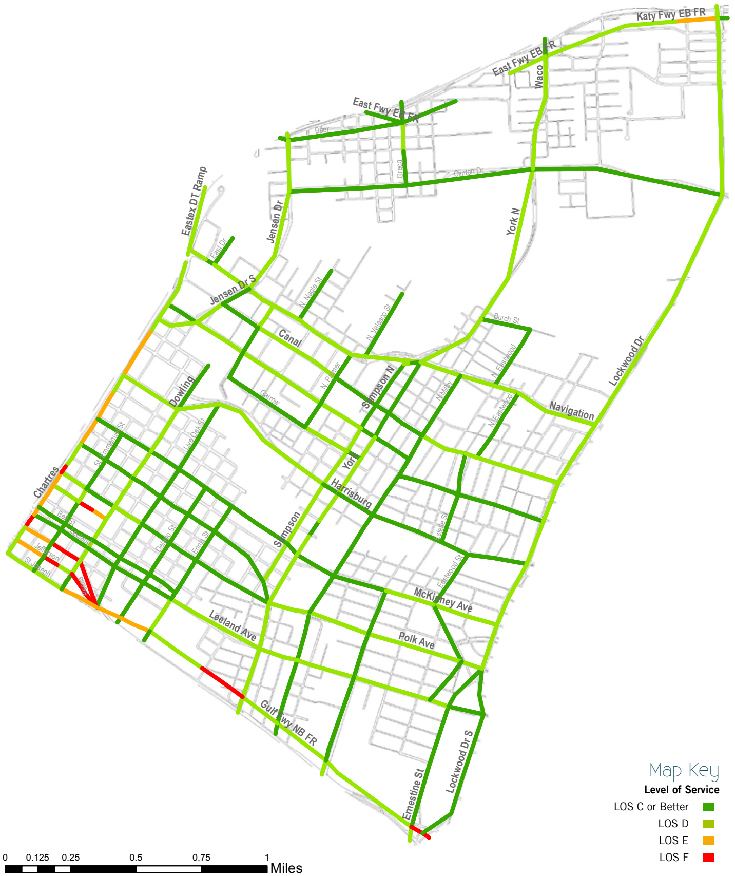
Figure ES1 Travel Demand Model Level of Service Analysis for 2035 Scenario 2: Master Plan/TOD
