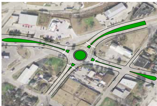
Figure 4.3 Conceptual Plan for Navigation Boulevard at York Street Roundabout
